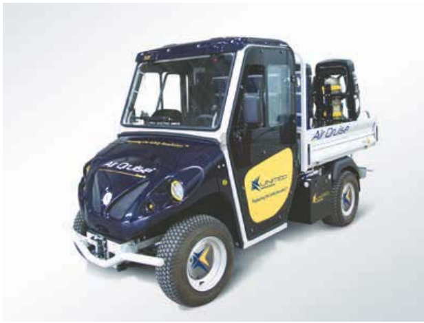
Figure 1. Driving the industry to safety. The Air Qruise™ Electro-Ex is an ATEX-certified explosion-proof vehicle equipped with a breathing air system that allows workers to drive safely through explosive and toxic environments.
